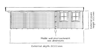
Use a flat level base allowing 100mm all around in addition to external cabin measurements
